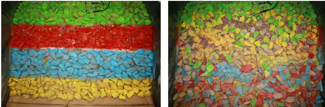
Figure 14 . Destruction of the type II RMB after the 3rd wave of 0.4 m.
