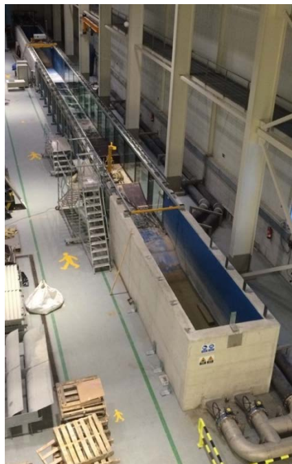
Figure 3. Tsunami-wave flume at IH Cantabria facilities in Santander. The test section in the middle of the flume has sides and bottom made of transparent glass.
