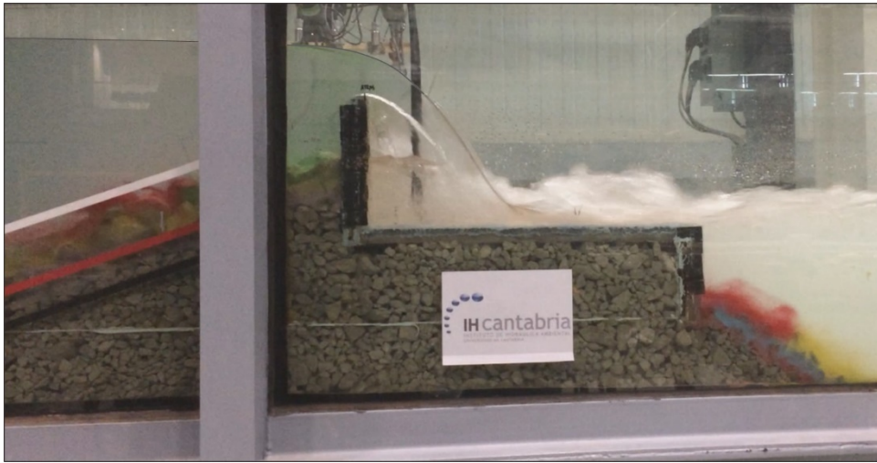
Figure 12 . Overflow current. Type I RMB. The overtopping flow falls on the horizontal plate.
