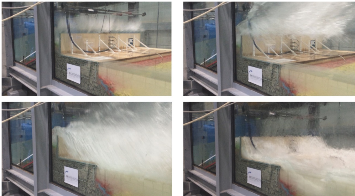
Figure 11. View of rubble-mound breakwater with crown wall (type I) under solitary wave test.
