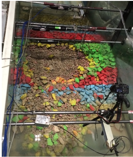
Figure 13. Top view of the type II model damage after overflow tests
