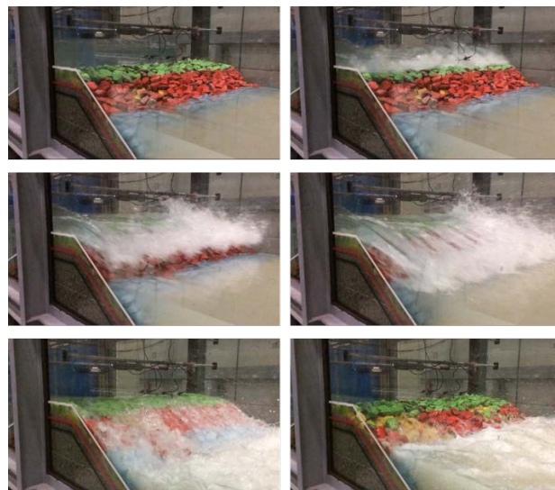
Figure 7. Lateral view of rubble-mound breakwater without crown wall (type II) under solitary wave test
