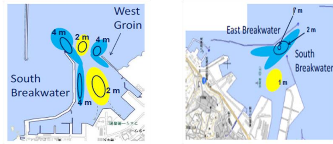
Figure 144: Hitachi Port (Left) and Oarai Port (Right) (dark blue: scour, yellow: accumulation) (PIANC, 2014).
