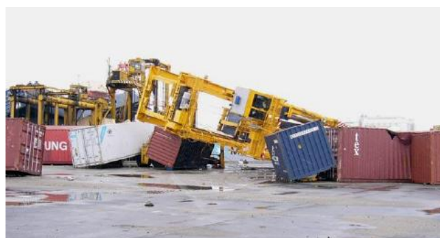
Figure 16: Damage to cargo handling machine at the container terminal of Sendai Shiogama Port (Photo courtesy: Y. Fukunaga).
