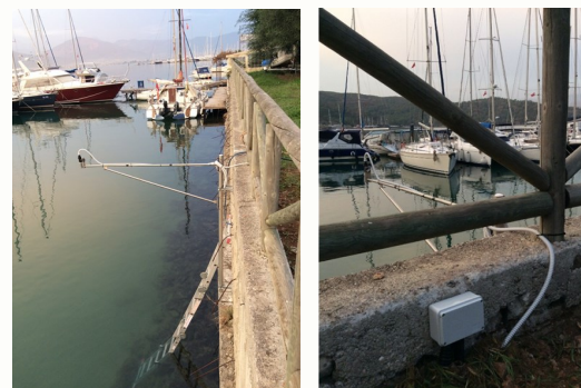
Left: The final position of IDSL with its sensor and pole. Right: The connection box between the sensor and the cable to the control panel including the temperature sensor inside.
